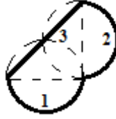
Fig. E2. Sketch to deduce the view factor F_{12} between two long hemicylinders (1) and (2).
