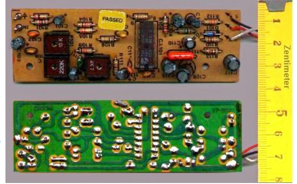
Fig. 1. a) Cross-section sketch of a PCB (about 1 mm thick). b) Example pictures of component-side and solder-side in a PCB.
