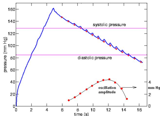
Fig. 16. Principle of oscillometric blood pressure measurement.
