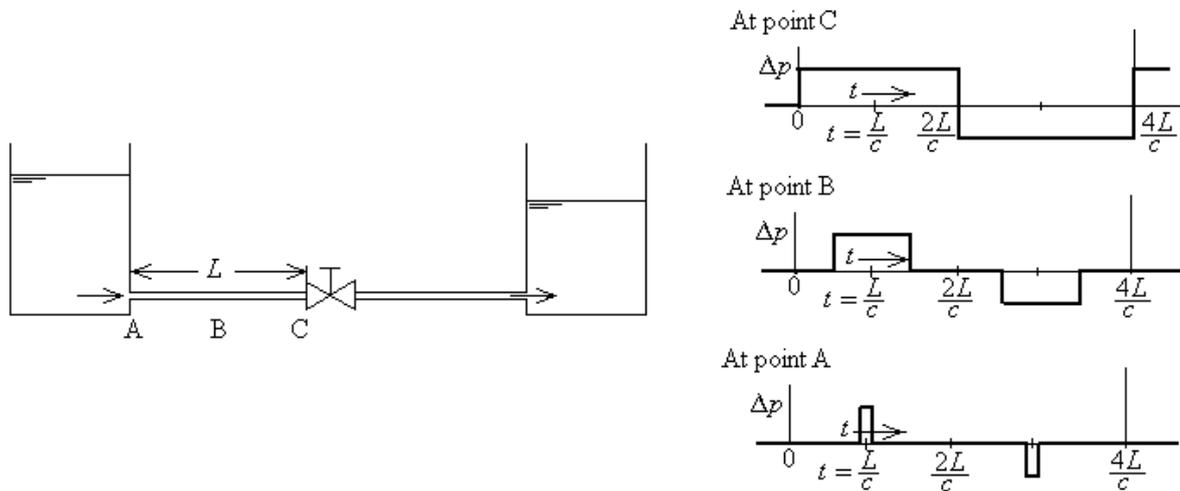
Fig. 7. Water hammer effect at different locations after valve closing at  $t=0$ .
