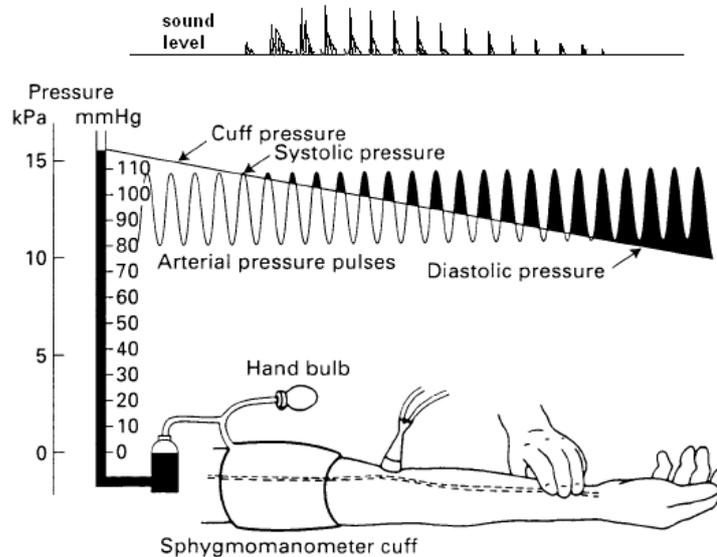
Fig. 15. Principle of auscultatory blood pressure measurement.
