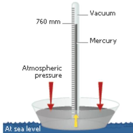
Fig. 2. Atmospheric pressure measurement (Torricelli's experiment).
