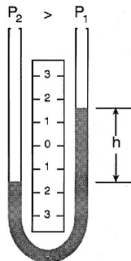
Fig. 10. U-tube manometer.
