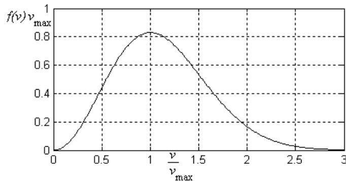
Fig. 4. Maxwell-Boltzmann distribution of molecular speeds at equilibrium.
